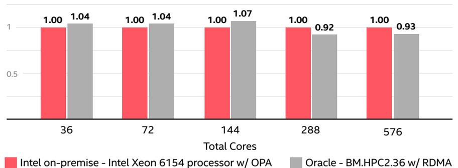
Figure 1. Relative performance results comparing LS-DYNA Car2Car model workload performance with scaling core counts of the Oracle BM.HPC2.36 and on-premises clusters.
