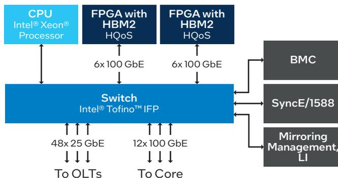
Figure 8. Example Intel® Tofino™ Expandable Architecture for OpenBNG.
