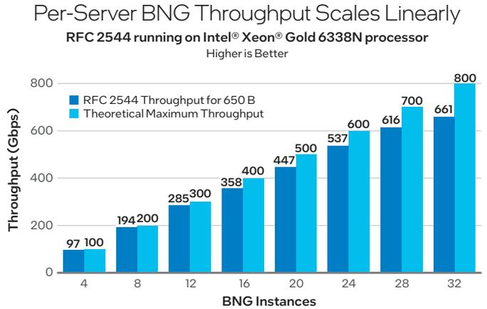
Figure 6. Linear scaling of vBNG throughput.<sup>4</sup>
