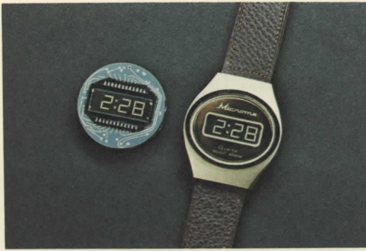
Microma sales in 1972 are represented by a solid-state quartz timekeeping module, as at left, and a finished quartz watch with liquid crystal display, as at right. The sale of modules to other watch manufacturers is expected to be a growing part of Microma business.
